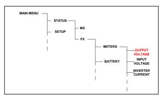
STATUS/FX/METERS------output 122 vac voltage DOWN UP TOP PORT
