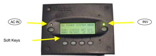
The MATE2M uses a six button user interface to navigate the menus and to change setpoints of various OutBack products.
