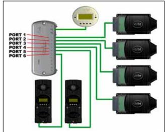
When first powering-up the system, make sure all of the OutBack products are plugged into the HUB and powered before plugging the MATE2M into the HUB.
